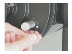
1.c. Using an Allen key remove the (3) screws that hold the collar and focusing mechanism in place. If the telescope has a mirror lock, unlock it to allow the mirror to be repositioned as needed when removing the focus knob and installing the FT Micro.
