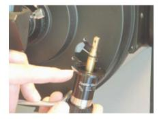
**2.a.** Locate the fillet on the Meade 8 Micro and position is so that this fillet rests next to the fillet of the back of the mirror cell. If it is not positioned as described the FTF Meade 8 Micro will not sit flush against the rear of the mirror cell.
