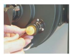
**3.d.** Replace the 3 Button Head Allen Screws and screw them in until they touch the flange of the Micro. Make sure that the Micro is seated properly and not cocked. If the unit is cocked some binding might result and it will not turn easily through it's travel. Once seated correctly tighten each screw more and more going from one screw to the next, this will improve the squareness of the Micro to the back of the mounting surface of the SCT.
