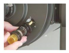
**3.b.** Slide the hole on the end of the Micro over the dowel on the mirror cell keeping the Micro as square as possible Push the mirror forward if needed to allow for a better angle when sliding the hole over the dowel.
