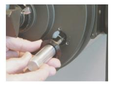
1.d. Remove the assembly by sliding the end of the focusing stem from the dowel by sliding it away from the center of the scope. If necessary rotate the knob CCW to extend the stem and push the mirror away from you to allow easier removal.
