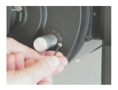
1.c. Using an Allen key remove the (3) screws that hold the collar and focusing mechanism in place. If the telescope has a mirror lock, unlock it to allow the mirror to be repositioned as needed when removing the focus knob and installing the FT Micro.
