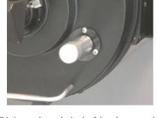
**1.b.** This image shows the back of the telescope and the focus knob that you will be replacing with the FT Micro.
