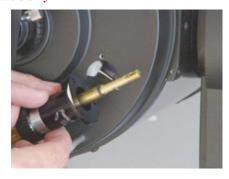
**2.b.** Unscrew the threaded part of the Micro to allow for more room when sliding the hole end of the Micro over the dowel pin on the mirror cell of the Meade SCT. You will feel an an abrupt change when you unscrew the stem at the end of it's internal travel.
