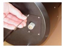
**1.a.** Place the telescope on a towel or a clean work surface and remove the (4) Phillips screws as shown.
