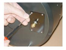
**2.d.** Attach the (4) Phillips screws as shown to the cover plate.
