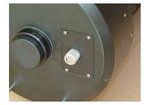
There are two different types of focus knobs on the C-9.25. If you have the one with the rubber focusing knob, remove the cover plate and then pull the rubber knob from the focusing nut. Be patient, these can sometimes be stuck and may take some coaxing to remove them. The rest of the instructions are the same for both models. If you have any difficulty feel free to contact us.
