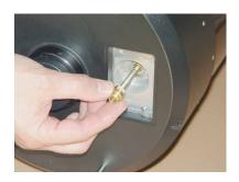
**2.a**. Screw the new focusing nut onto the stem as shown.
