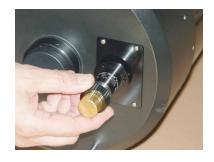
**2.g.** Position the Micro so that the holes in the Micro align with the holes on the cover plate.
