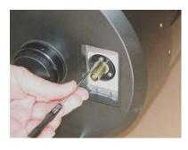
**1.e**. Loosen and remove the (3) Phillips screws that hold the bearing cover housing.
