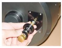
**2.e**. Screw the focusing nut onto the end of the Feather Touch Micro until snug.
