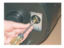
**1.d.** Remove the Phillips screw from the focusing stem as shown.
