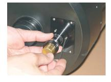
**2.h.** Use the 4-40 Allan head screws to fasten the Micro to the cover plate.
