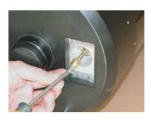
**2.b.** Reattach the Phillips screw onto the focusing stem as shown. <u>IMPORTANT:</u> This screw secures the mirror assembly and must be reattached to prevent the mirror from falling forward if the focusing knob is unscrewed all the way.
