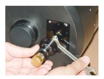
**2.f.** Hold the unit as shown on the black coarse focusing knob and tighten the nut onto the Micro with an open end wrench.
