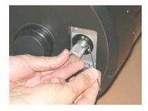
**1.c.** With an Allen key loosen the set screw to remove the focus knob as shown.
